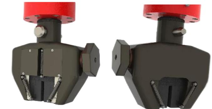
Special fixture of biaxial testing machine tensile
