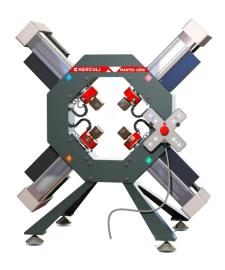
The Mantis series Tabletop biaxial testing machine has a load range of 1KN to 50KN. It features remarkable high precision and efficiency. It can precisely test various properties of materials under biaxial stress conditions, including key indicators such as strength, deformation, and failure, offering valuable experimental data for product development,
